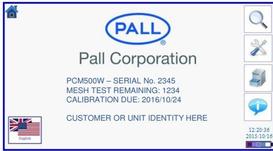
The main menu includes PCM500 serial number, mesh test detail, calibration date, and customer or unit identity if installed.
