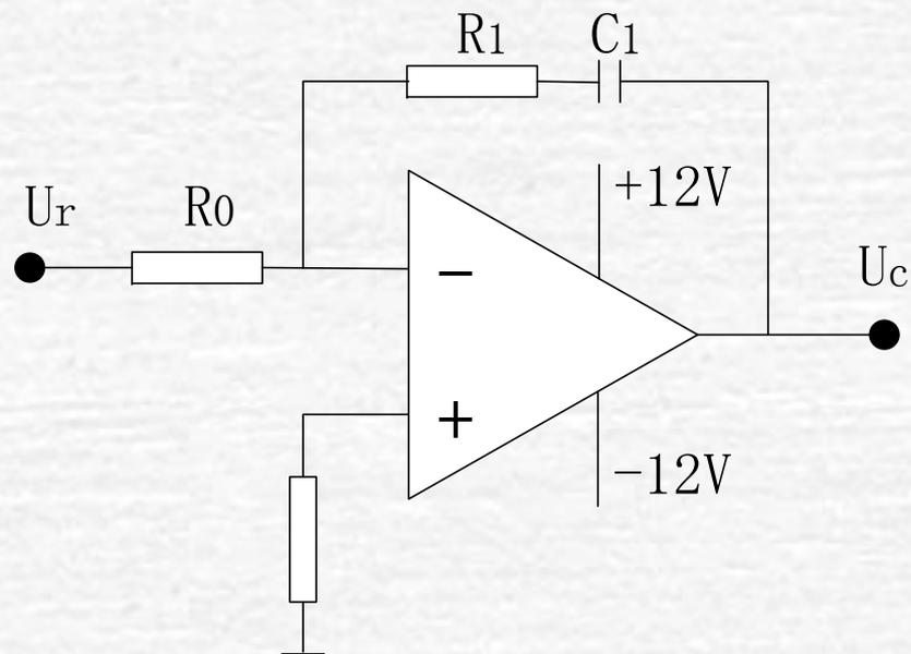
$$\frac{U_c(s)}{U_r(s)} = -\frac{R_1 C_1 s + 1}{R_0 C_1 s}$$
