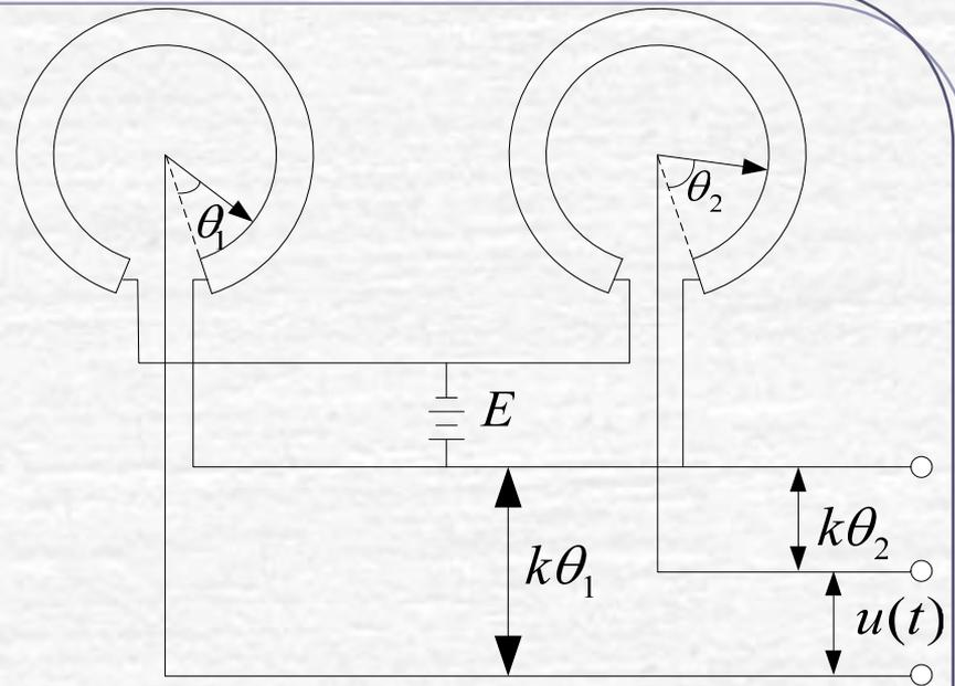
$$\begin{aligned} u(t) &= u_1(t) - u_2(t) = K_p (\theta_1(t) - \theta_2(t)) \\ &= K_p \Delta\theta(t) \end{aligned}$$
