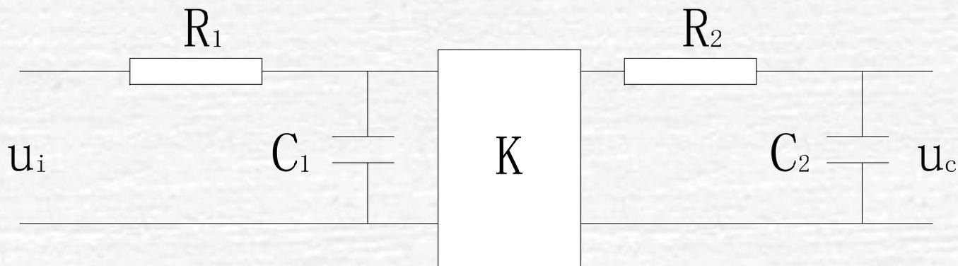
$$\frac{U_c(s)}{U_i(s)} = \frac{K}{(R_1 C_1 s + 1)(R_2 C_2 s + 1)}$$
