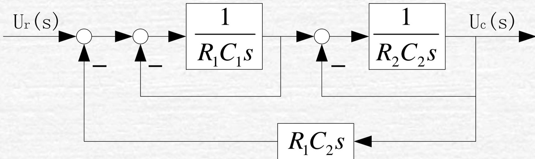
$$\frac{U_c(s)}{U_r(s)} = \frac{1}{(R_1 C_1 s + 1)(R_2 C_2 s + 1) + R_1 C_2 s}$$
