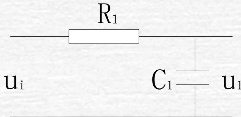
$$\frac{U_1(s)}{U_i(s)} = \frac{\frac{1}{sC_1}}{R_1 + \frac{1}{sC_1}} = \frac{1}{R_1C_1s + 1}$$
