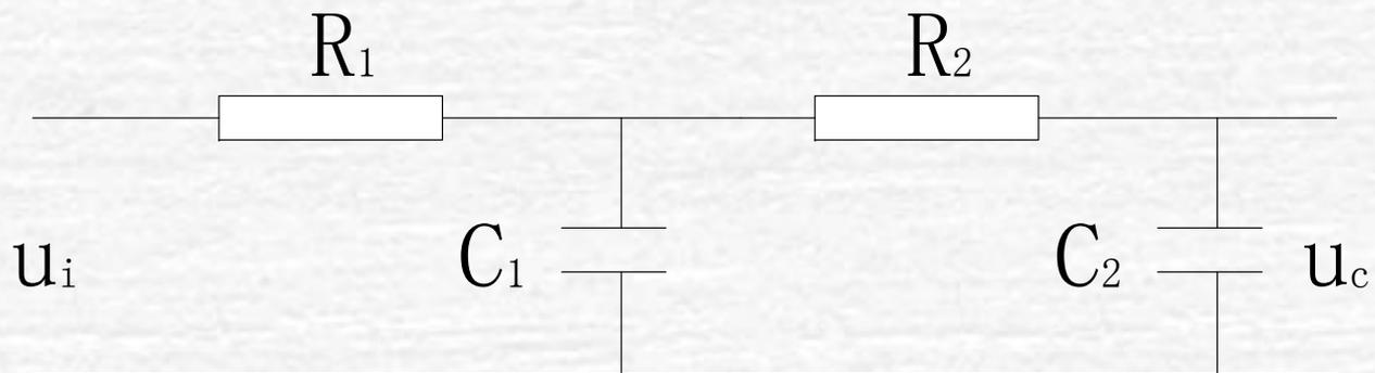
$$\frac{U_c(s)}{U_i(s)} = \frac{1}{R_1 R_2 C_1 C_2 S^2 + (R_1 C_1 + R_1 C_2 + R_2 C_2) s + 1}$$
