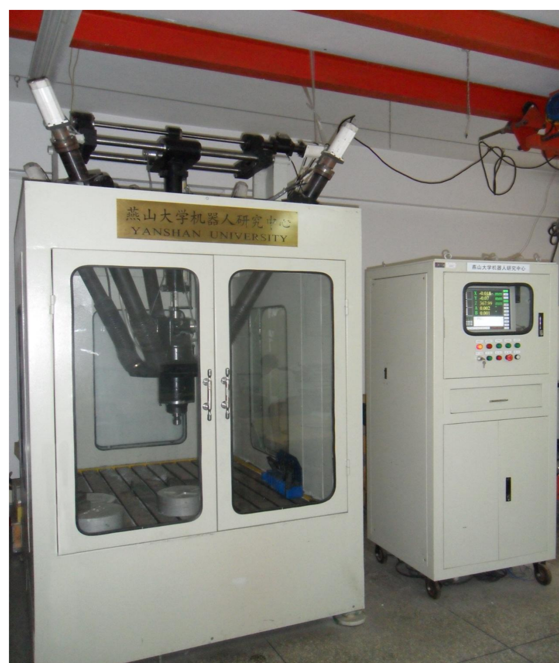
图2 5-UPS/PRPU并联机床
